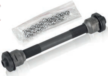
216 95 01000 9895 repair kit with axle, bearing rings, end caps
